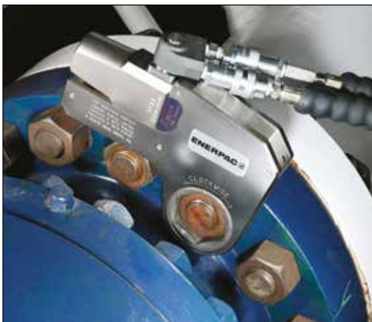
◀ The ZE4T-Series torque wrench pumps are perfectly matched for this W2000X wrench.
