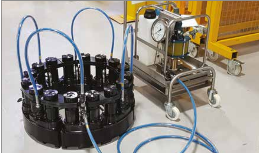
▲ Multi Stud Tensioning Set-Up.
