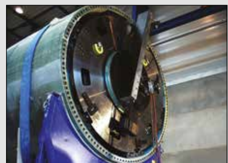
▲ Orbital milling machines for wind turbine manufacture.
