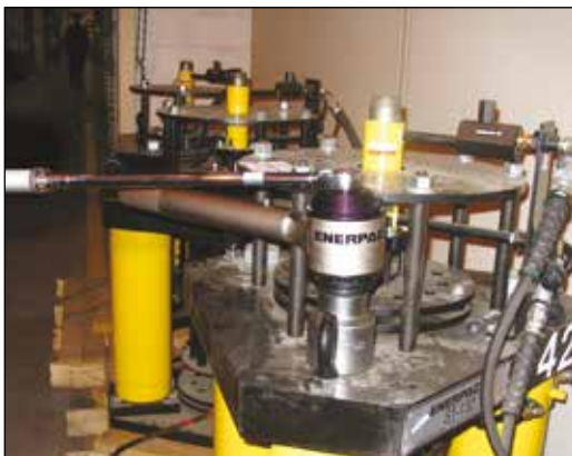
◀ Enerpac Reaction Bar Torque Multiplier E393 used to manually torque bolts up to 4300 Nm.
