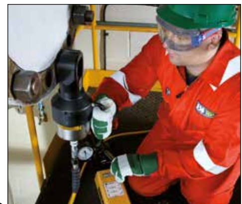
Nut splitter set for joint separation during inspection, maintenance and decommissioning operations. ▶
