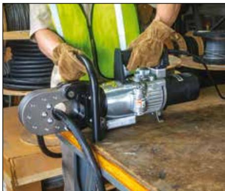
◀ Cut through wire rope and cables with ease.
