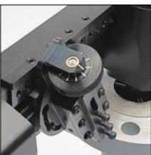
Tool bit fine depth adjustment.
